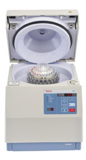
A new automated, high-performance cell washer has been recently announced by Thermo Fischer Scientific. It is specifically designed to enable precise, thorough, reproducible and rapid blood cell washing of up to 24 tubes in a three-minute run.
