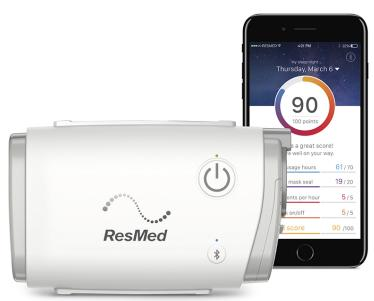
ResMed, one of the bigger names in CPAP (continuous positive airway pressure) therapy, has unveiled the world's smallest CPAP device. The ResMed AirMini weighs less than 11 ounces (300 grams) and is only 5.4 inches (14 cm) on its longest side. Being so light and small can help patients take it along when traveling, as traditional full size CPAP devices are impractically large.
