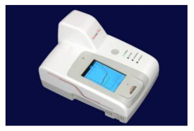
Innovation comes in all sizes. Bigtec's mini PCR, TrueLab, is the perfect example for that. TrueLab is a point-of-care, handheld, real time quantitative mini PCR, that is battery operated. This device that can easily be lifted in one hand detects the disease organism by a polymerase chain reaction carried out on a chip that is designed using MEMS (Microelectromechanical systems) technology and is specific to each disease.
