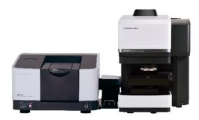
Shimadzu will launch a particle analysis system in Japan and overseas, specialising in the analysis of microplastics, at global scale. This system can quickly calculate the number of particles, area, volume, mass, and individual particle qualities of microplastics based on the measurement results from an infrared microscope or an infrared Raman microscope.
