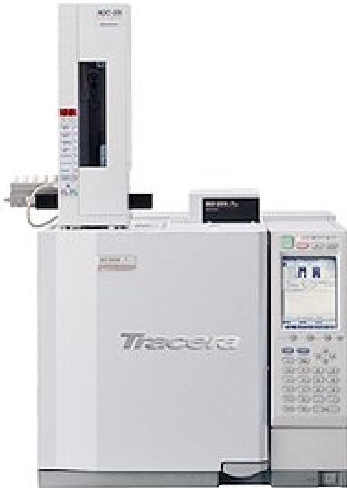
**Singapore:** Shimadzu will introduce Tracera, a high-sensitivity gas chromatograph equipped with the newly developed barrier discharge ionization detector (BID), which is capable of detecting all types of trace organic and inorganic compounds, with the exception of helium (He) and neon (Ne), at the 0.1 ppm level.
