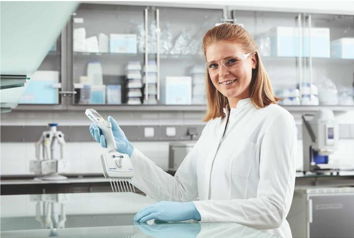
The new electronic Eppendorf Xplorer® plus Move It® models feature 8 or 12 channels and volume ranges of 1–20 µL or 5–100 µL respectively. With a minimum tip distance of 4.5 mm they are perfectly suited for the 384-well plate format.
