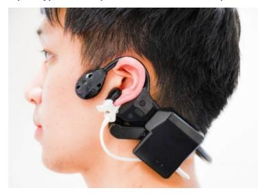
Kyocera Corporation and Tokyo Medical and Dental University (TMDU) announced a joint research project to develop a wireless headset that can remotely monitor high accuracy patient biometrics, such as blood oxygen saturation (SpO2). The Department of Cardiovascular Medicine of TMDU Medical Hospital began preparing for clinical research of the wearable headset system in May 2020.
