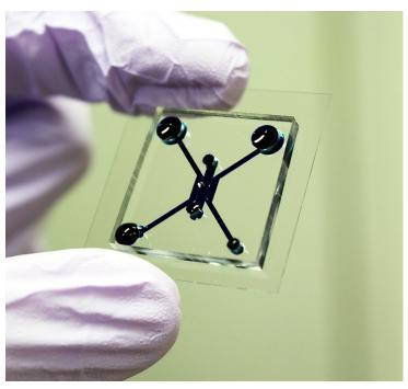
Kyoto University researchers have developed a new 'tumor-on-a-chip' device that can better mimic the environment inside the body, paving the way for improved screening of potential cancer fighting drugs.
