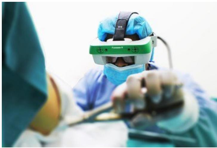
Foresee-X is a set of smart surgical glasses with functionality based on augmented reality (AR) and mixed reality technologies. This device was developed by SURGLASSES, also known as Taiwan Main Orthopaedic Biotechnology Co. Ltd., and has received IEC60601-1-2 and ISO 13485 certifications. It is designed to bring a higher level of support to surgical procedures for trauma cases.
