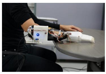
The Biological Systems Engineering Lab at Hiroshima University, Japan has developed a new 3D printed prosthetic hand combined with a computer interface, which is their cheapest, lightest model that is more reactive to motion intent than before. Previous generations of their prosthetic hands have been made of metal, which is heavy and expensive to make.
