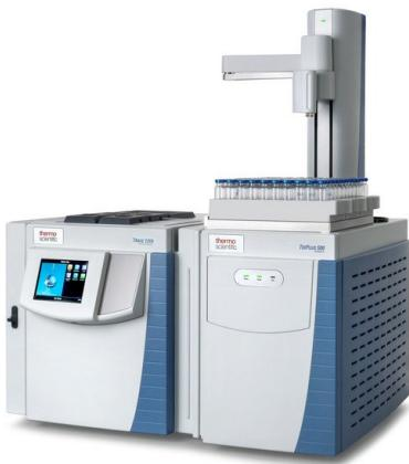
The Thermo Scientific TriPlus 500 Gas Chromatography Headspace Autosampler is designed for high sample throughput and low cost-per-sample for routine Volatile Organic Compounds (VOCs) analysis by pharmaceutical, food safety and environmental scientists. Thermo Fisher Scientific is showcasing its new system during the 2019 Pittsburgh Conference & Exposition (Pittcon 2019), being held March 17-21, at the Pennsylvania Conference Center, Philadelphia.
