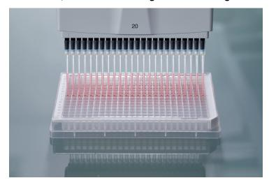
With their 16 and 24 channels, the new mechanical multichannel pipettes Eppendorf Research plus and the new electronic multichannel pipettes Eppendorf Xplorer plus can now tackle entire columns and rows of a 384-well plate in one single step. Up to 24 reactions may thus be started and stopped simultaneously. An entire plate can be managed manually within the space of a minute. In this way, the user will save time while at the same time improving the reproducibility of their results.
