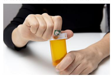
In new research IBM team details a first-of-a-kind "fingernail sensor" prototype to help monitor human health. The wearable, wireless device continuously measures how a person's fingernail bends and moves, which is a key indicator of grip strength.
