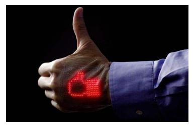
A group of researchers, at the University of Tokyo's Graduate School of Engineering in collaboration with Dai Nippon Printing, a leading Japanese printing company, has developed an ultrathin, highly elastic skin display device that can show the moving waveform of an electrocardiogram recorded by a breathable, on-skin electrode sensor.
